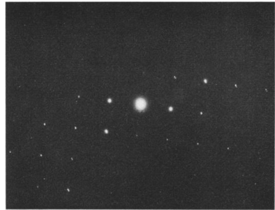
Figure 12 Selected-area diffraction pattern (700 keV) from a grain-boundary domain in stoichiometric CuPt ordered 14 h at 550°C. Note doubling of many spots, indicating that selected area encompasses two ordered orientation variants. This SADP includes no superlattice spots.
