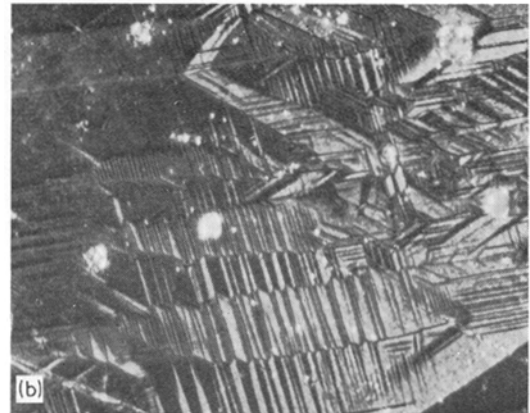
Figure 16 Stoichiometric CuPt, thermally polished at 900°C, quenched and ordered for (a) 23 h at 350°C, (b) 228 h at 475°C. Viewed under polarized light (a) \times 54 , (b) \times 108 .
