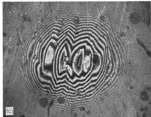
Figure 17 Stoichiometric CuPt, thermally polished at 900°C and continuously cooled at 3°C h -1 to about 300°C. (a) and (b) viewed by polarized light; \times 190 . (c) Multiple-beam interferogram, showing surface tilts associated with macrotwins shown in (a) above \times 100 .
