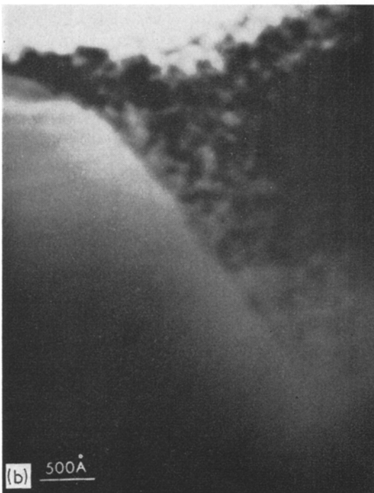
Figure 11 Electron-micrographs (700 keV) of stoichiometric CuPt, ordered at 550°C for 14 h. (a) Matrix with fine ordered/disordered two-phase structure. (b) Matrix plus ordered grain-boundary domains. Marker = 0.2 μm. (Inset shows corresponding SADP, which includes both fundamental and superlattice spots.)
